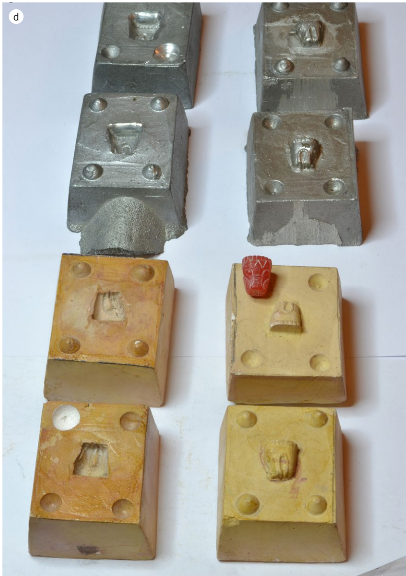
d) Left and right plaster moulds for the metal formers (top) for the leonine protome e) Tube: left and right plaster moulds produced from a clay model of the tube f) Tube: left and right metal formers cast from the plaster moulds - fig. 12e
